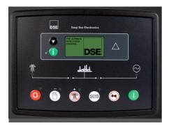
The DSE6120 is an Auto Start & Auto Mains (Utility) Failure Control Module suitable for a wide variety of single, diesel or gas, gen-set applications. It monitors speed, frequency, voltage, current, oil pressure, coolant temperature and fuel level, and the modules will display warnings, shutdown and engine status information on the backlit LCD screen and illuminated LED.
